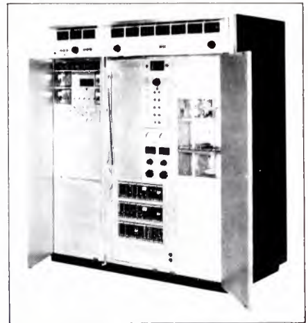
The automatic TT-25FL VHF Lowband Transmitter.
