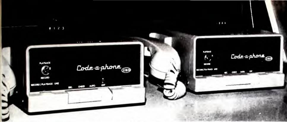
Two Code-a-phone Model 250 units. Connected to telephones on weekends, a call to one records a vote for one "contestant;" a call to the other for the opponent. Count is kept by automatic counters shown here on top of machines and connected to them.
